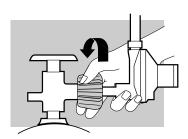
Note: This is a new type of connection. It tightens clockwise and will not allow gas to flow unless the connection is tight. The connection requires tightening by hand only.
